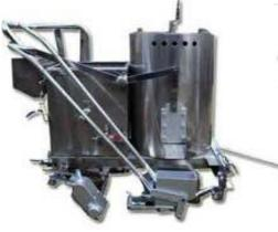
SS 2 Layer Type Tank 4 Bags / 100 kg capacity 10" Rubber Wheel Chain Drive Type Bead Dispenser
